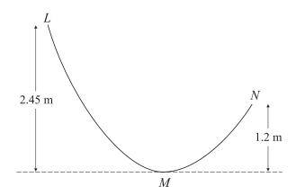
The diagram shows the vertical cross-section LMN of a fixed smooth surface. M is the lowest point of the cross-section. L is 2.45 m above the level of M, and N is 1.2 m above the level of M. A particle of mass 0.5 kg is released from rest at L and moves on the surface until it leaves it at N. Find
