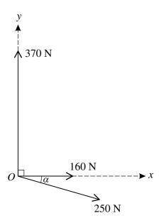
Coplanar forces of magnitudes 250 N, 160 N and 370 N act at a point O in the directions shown in the diagram, where the angle  $\alpha$  is such that  $\sin \alpha = 0.28$  and  $\cos \alpha = 0.96$ . Calculate the magnitude of the resultant of the three forces. Calculate also the angle that the resultant makes with the x-direction.
