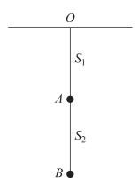
$S_1$  and  $S_2$  are light inextensible strings, and A and B are particles each of mass 0.2 kg. Particle A is suspended from a fixed point O by the string  $S_1$ , and particle B is suspended from A by the string  $S_2$ . The particles hang in equilibrium as shown in the diagram.
