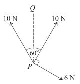
Three coplanar forces of magnitudes  $10 \,\mathrm{N}$ ,  $10 \,\mathrm{N}$  and  $6 \,\mathrm{N}$  act at a point P in the directions shown in the diagram. PQ is the bisector of the angle between the two forces of magnitude  $10 \,\mathrm{N}$ .
