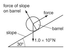
A force is applied to the barrel to move it up the slope at constant speed. The force is parallel to the slope.
