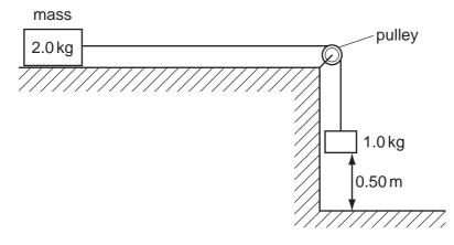
What is the speed of the 2.0 kg mass as the 1.0 kg mass hits the floor, having fallen a distance of 0.50 m?
