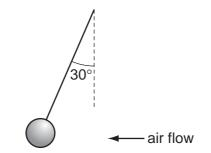
The ball is suspended by a light string and weighs 0.15 N.
