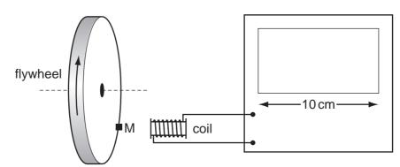
The flywheel has a small magnet M mounted on it. Each time the magnet passes the coil, a voltage pulse is generated, which is passed to the c.r.o. The display of the c.r.o. is 10 cm wide. The flywheel is rotating at a rate of about 3000 revolutions per minute.
