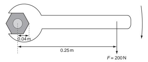
A force F is applied at right-angles to the spanner at a distance of 0.25 m from the centre of the nut. When the nut is fully tightened, the applied force is 200 N.
