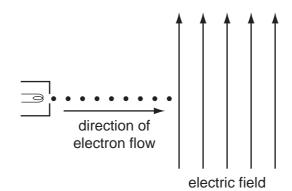
An electron gun injects a beam of electrons horizontally into the field.
