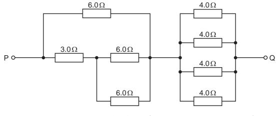
What is the resistance between the points P and Q due to the resistance network?
