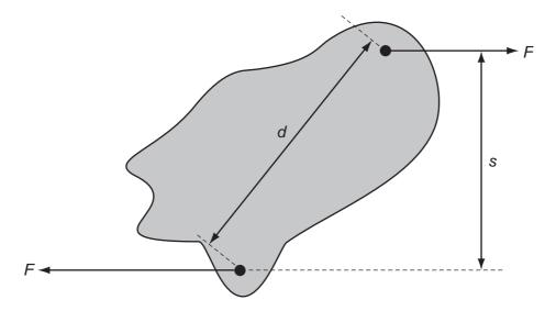
What is the magnitude of the torque on the body produced by these forces?
