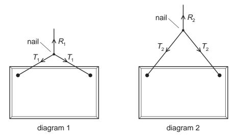
In both cases, a string is attached to the same points on the picture and looped symmetrically over a nail in a wall. The forces shown are those that act on the nail.
