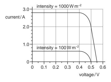
At zero voltage, what is the ratio  $\frac{\text{current at } 1000 \, \text{W m}^{-2}}{2}$ ?
