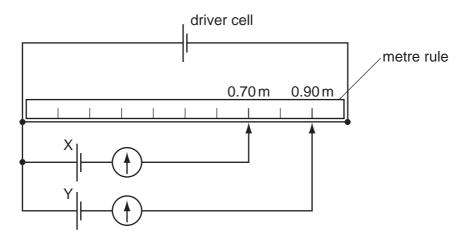
The balance points for cells X and Y are 0.70 m and 0.90 m respectively.
