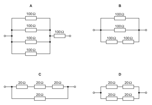
**37** Which circuit has a resistance of  $40\Omega$  between the terminals?
