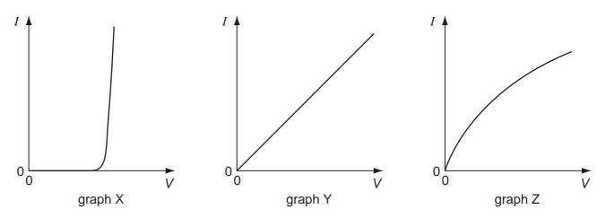
The components are a metal wire at constant temperature, a semiconductor diode and a filament lamp.
