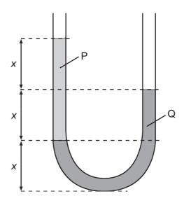
What is the ratio  $\frac{\text{density of P}}{\text{density of Q}}$ ?
