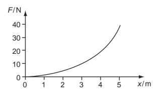
The energy stored in the rubber for an extension of 5 m is
