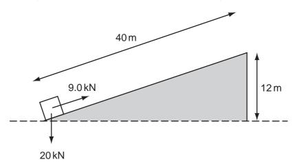
How much of the work done is dissipated as heat?
