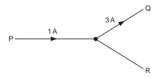
How many coulombs of charge pass a given point in wire R in 5 seconds?
