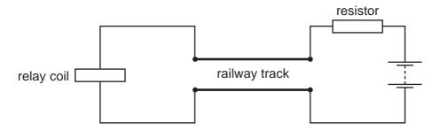
With no train present, there is a current in the relay coil which operates a switch to turn on a light.
