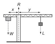
A mass provides a balancing load W. The position of the load is such that the system is perfectly balanced with Wx = Ly. The ground provides a reaction force R. The distance x does not change.
