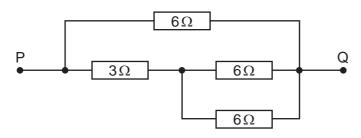
What is the resistance between the points P and Q due to the resistance network?
