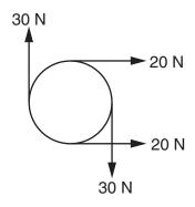
Which of the following describes the resultant force and resultant torque on the object?
