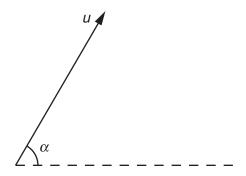
What will be the vertical and horizontal components of its velocity after a time t? Assume that air resistance is negligible. The acceleration of free fall is g.
