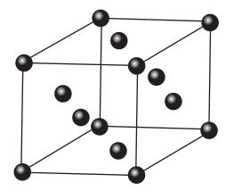
The particles present in such a crystal may be atoms, molecules, anions or cations. In the diagram above, the particles present are represented by ...
