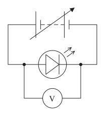
He increased the potential difference V from zero and recorded the value at which the LED just began to emit light. He repeated this for LEDs that emitted light of different, known frequencies f.
