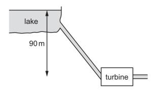
The mass flow rate of the water is 2400 kg min<sup>-1</sup>. The turbine has an efficiency of 75%.
