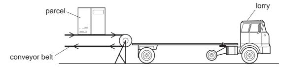
The parcel travels towards the lorry at a constant speed. Only two horizontal forces act on the parcel: air resistance, and friction with the conveyor belt.
