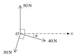
Coplanar forces of magnitudes 50 N, 40 N and 30 N act at a point O in the directions shown in the diagram, where  $\tan \alpha = \frac{7}{24}$ .
