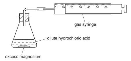
The volume of hydrogen produced was measured every minute for six minutes.
