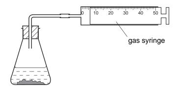
Solids **W** and **X** both catalyse the breakdown of hydrogen peroxide. The syringe diagrams show the volume of oxygen formed every 20 seconds using these catalysts at 25 °C.
