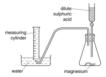
In an experiment 50 cm<sup>3</sup> of dilute sulphuric acid was added to a large piece of magnesium. A student measured the total volume of gas produced at 2 minute intervals.
